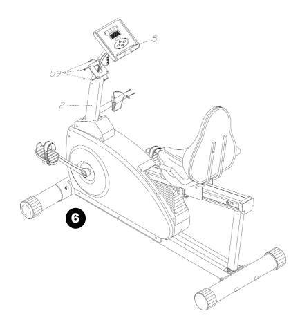
**6.** Connect the computer cable at the top of the console tube (2) to the console (5). Both computer cable connections have white ends. Feed the pulse wires from the console (5) down into the console tube (2) and out the rear hole in the handlebar area. Attach the console tube (2) to the console (5) with the screws (59) provided and already attached to back of the console (5). Attach bottle rack to console tube (2).
